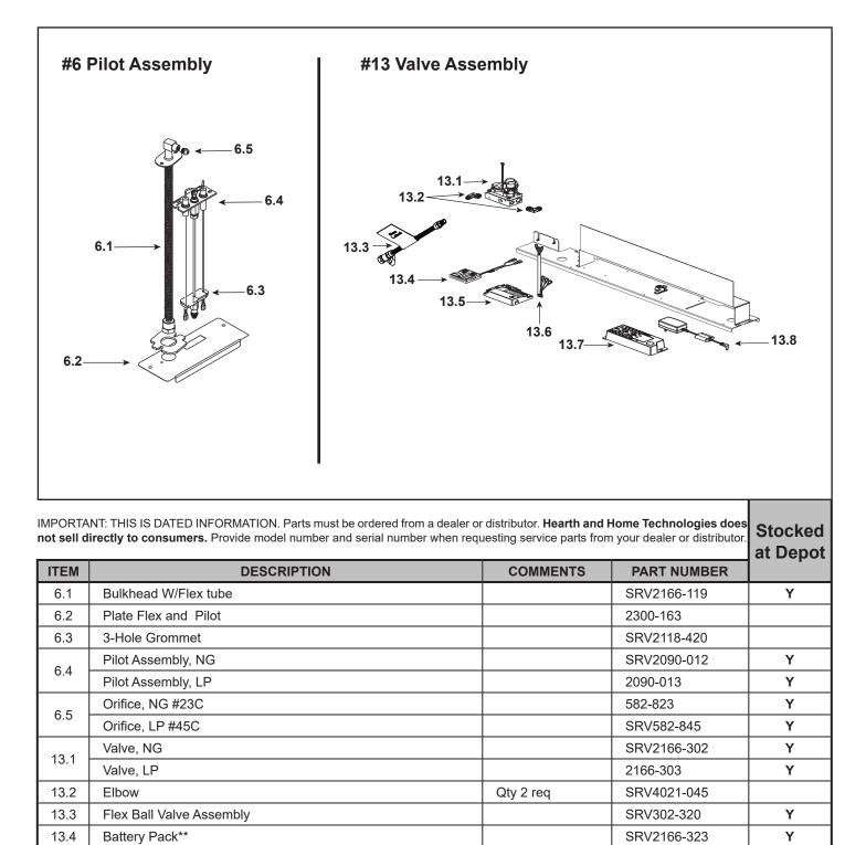
\*\*Fuse for battery pack can be sourced locally, not a warranty item. Specs are 250v, 1A fuse, 3/4" long Additional service part numbers on following page.
