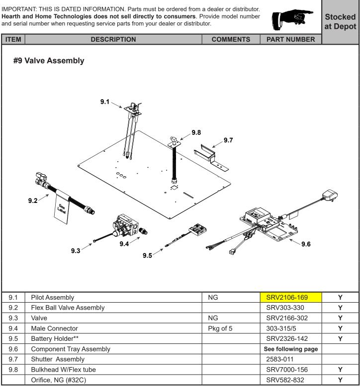
\*\*Fuse for battery pack can be sourced locally, not a warranty item. Specs are 250v, 3A fuse, 3/4" long Additional service part numbers on following page.
