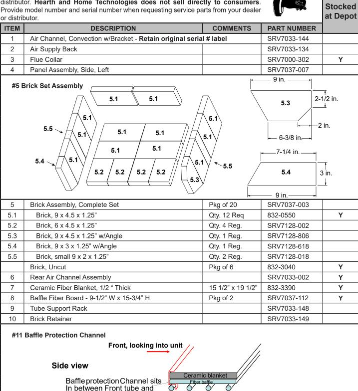
**Baffle Protection Channel** SRV7033-298 11
