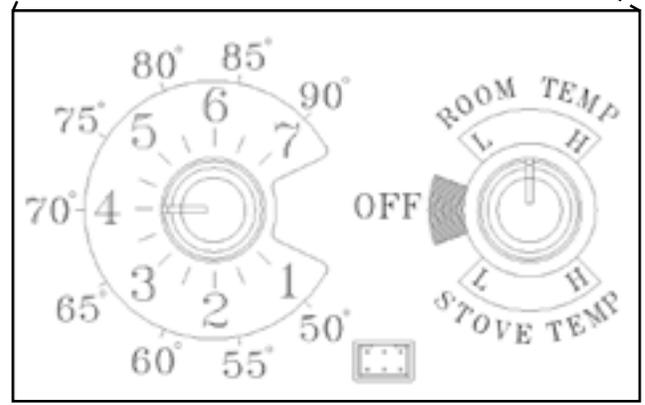
**Room Temperature Mode:** This setting, see above, will produce a room temperature of 70 degrees with the distribution blower at medium speed.
