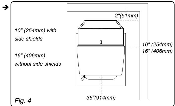
Minimum Size floor protection (USA) is 32<sup>1/2</sup>" wide By 33" deep (825mm X 838mm).
