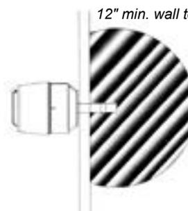
36" min clearance to any combustible material
