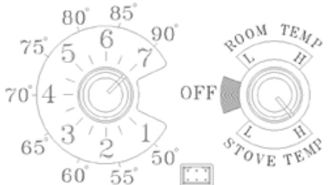
*The setting above will produce continuous maximum heat output with the distribution blower at full speed.*
