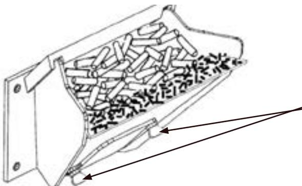
Loosen these two wing screws for access to clean the air passage and igniter.
