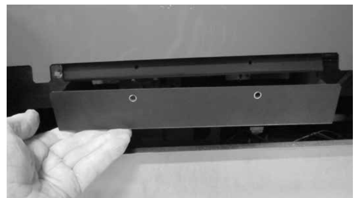
Figure 4.16 Removal of Air Chamber Cover
