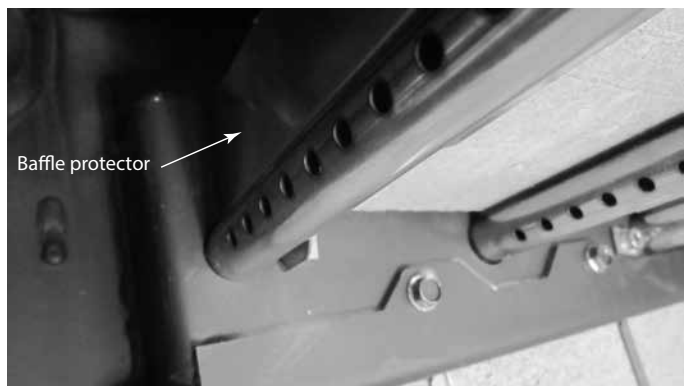
Figure 4.9 Reinstall Baffle Protection Channel
