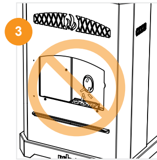
3 Auger stops feeding pellets.
