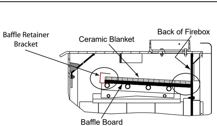
Ceramic Blanket and Baffle Board **MUST** be in contact with the back of the firebox and even with each other in the front.
