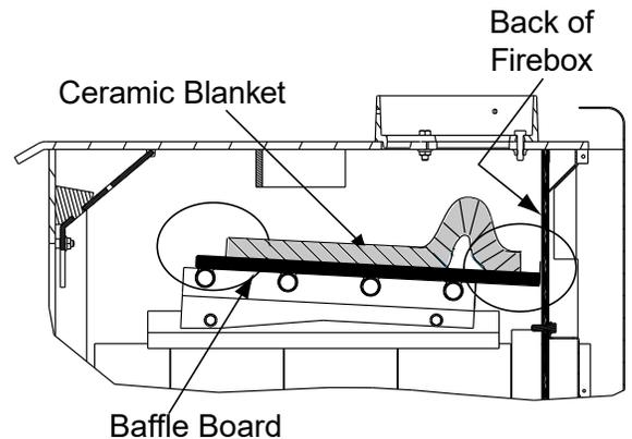
Ceramic Blanket is bunched up at the back of the firebox and **NOT** even with the Baffle Board in the front.
