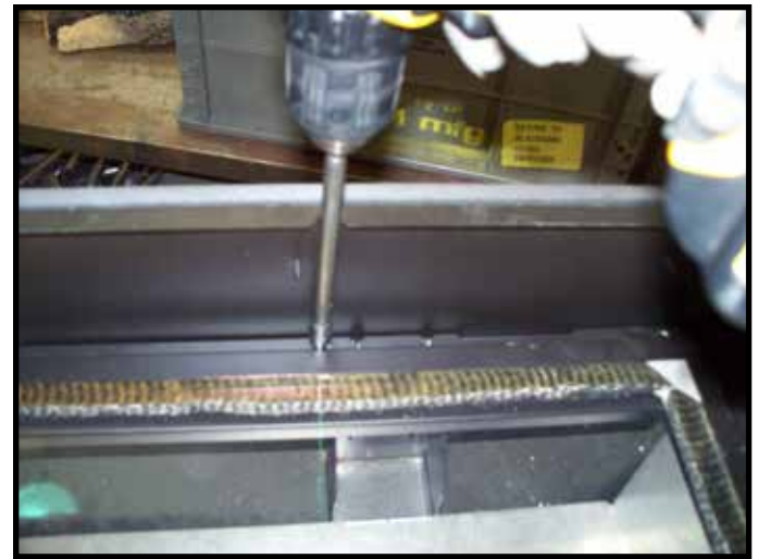
Figure 9.4. Gas and Electrical Access - Remove Glass Window
