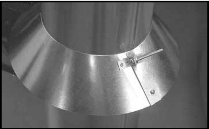
Figure 7.11 Insert Bolt into Brackets
