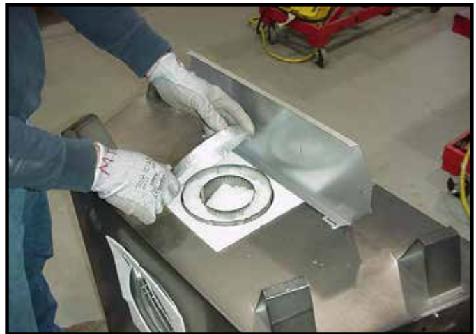
Figure 6.4 Remove the seal cap.
