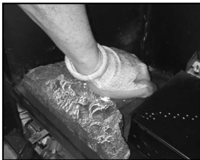
Figure 11.2 Press Left Hearth Firmly Into Place
