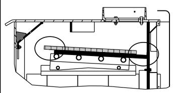
Ceramic Blanket is NOT in contact with the back of the firebox and NOT even with the Baffle Board in the front.
