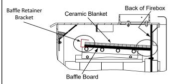
Ceramic Blanket and Baffle Board MUST be in contact with the back of the firebox and even with each other in the front.
