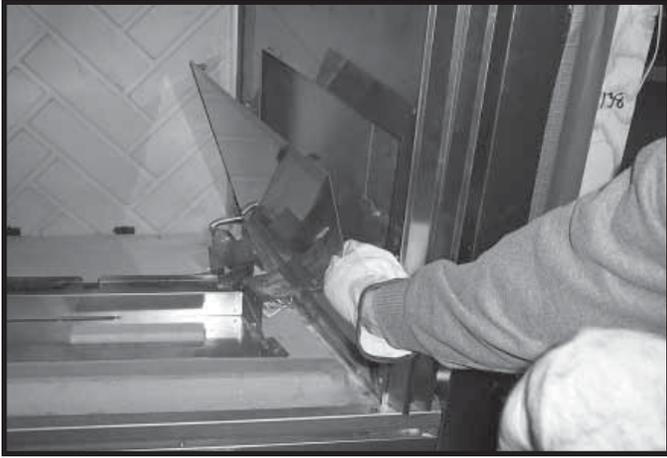
Figure 10. Remove Valve Access Panel
