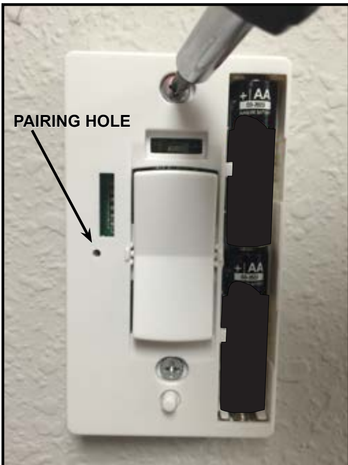
Figure 3. Mounting IFT-RC150 Wireless Wall Switch
