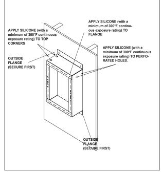
Figure 2.10 HEAT-OUT-BEK Attached to Wall
