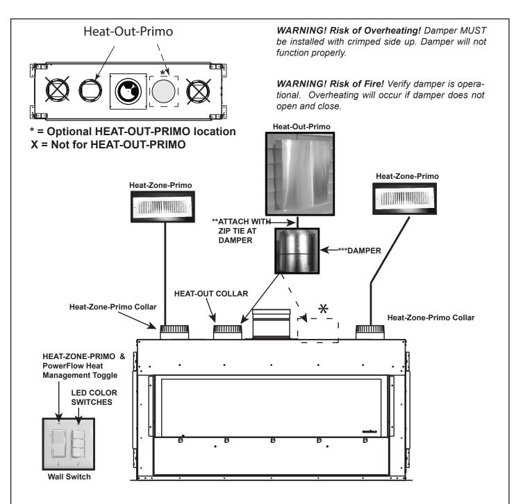
\*The Heat-Out-Primo may be installed in either position shown above.
