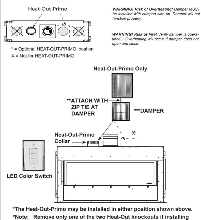
\*Note: Remove only one of the two Heat-Out knockouts if installing the HEAT-OUT-PRIMO. The other knockout must remain installed. \*\* Use included zip ties to attach the flex duct to the damper. \*\*\*Verify damper is operational and no obstructions, such as screws, are present.
