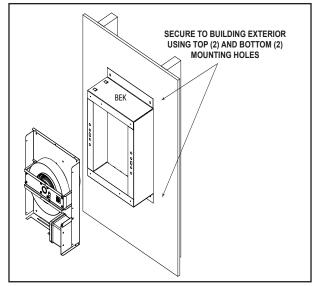
Figure 2.12 HEAT-OUT-PRIMO Attached to HEAT-OUT-BEK
