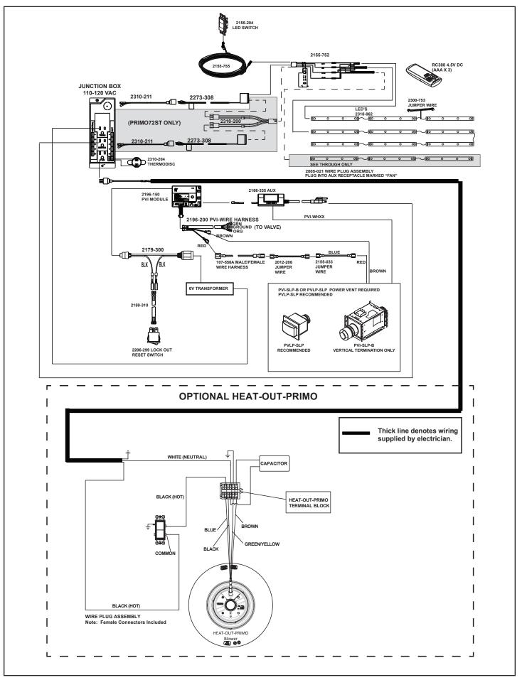
Figure 3.4 Passive Heat with HEAT-OUT-PRIMO
