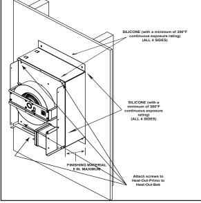
Figure 2.13 Silicone Weather Sealing
