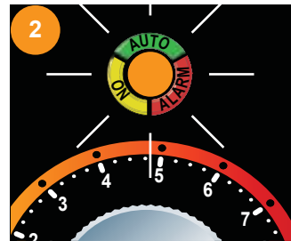
2 LED light will flash amber rapidly *Early models may have a green continuous blinking light during shutdown sequence.
