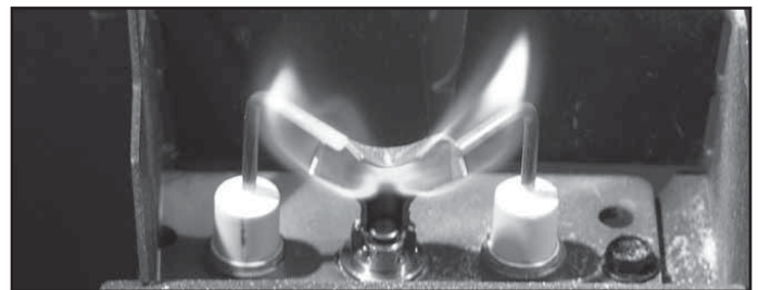
Figure 3.1 IPI Pilot Flame Patterns
