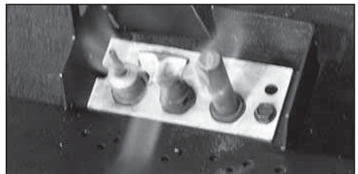
Figure 3.2 Standing Pilot Flame Patterns
