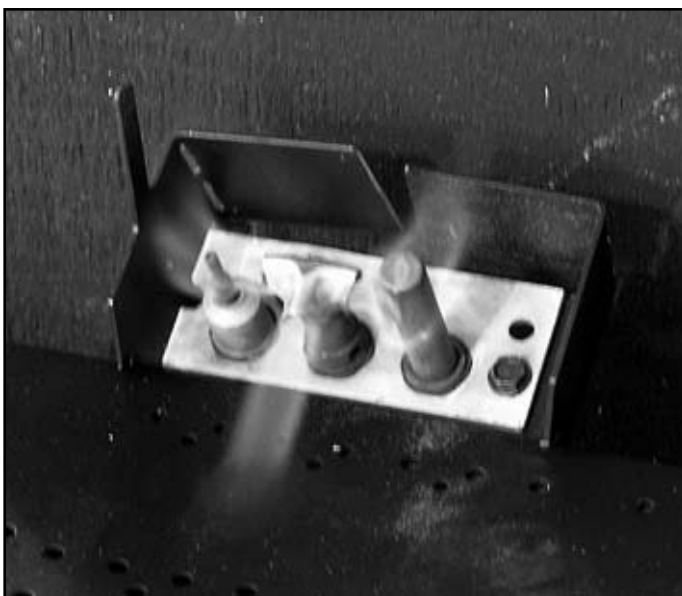
Figure 3.2 Standing Pilot Flame Patterns
