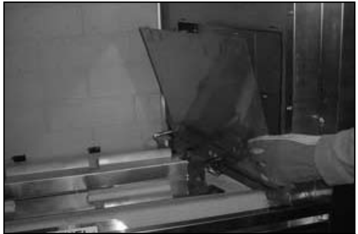
Figure 11.4 Remove Valve Access Panel
