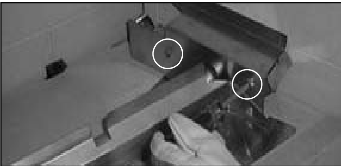
Figure 11.2 Remove Pilot Shield
