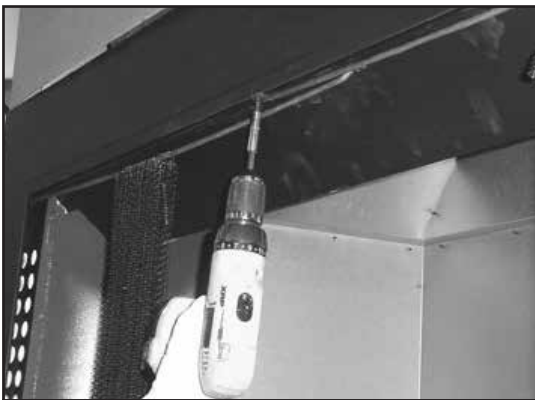
Figure 3.8 Remove Screen Rods
