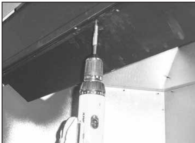
Figure 8.1 Remove Smoke Shield
