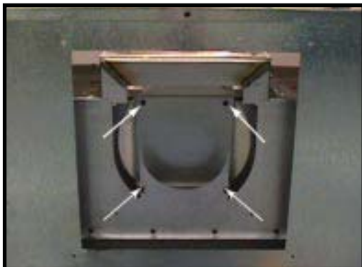
Figure 12 - Remove Inner Cover Plate
