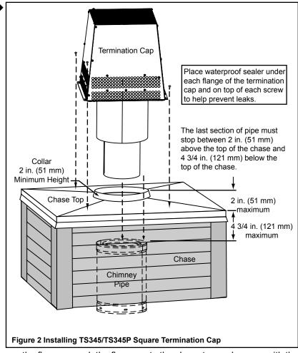
the flanges, push the flange onto the chase top and secure with the four screws provided in the fastener package. Place a small dab of waterproof sealant over each screw head to ensure a leak tight top.
