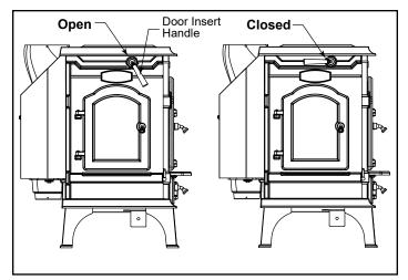
Figure 27 - Damper operating positions.
