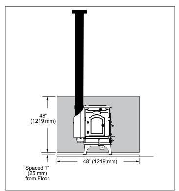
Figure 17 - Sidewall protection.
