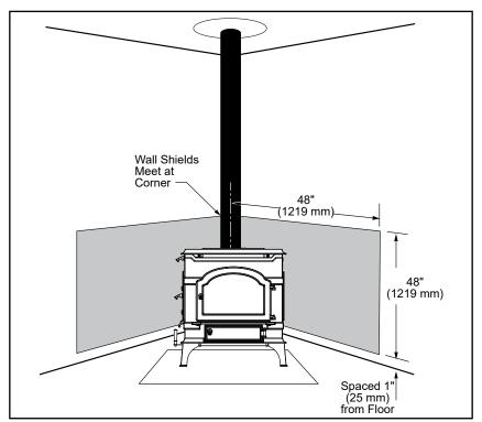
Figure 18 - Corner wall protection.
