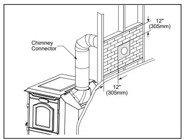
Figure 10 - Wall pass-through enclosed with noncombustible materials.
