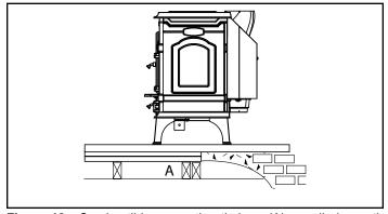
**Figure 13** - Combustible supporting timbers (A) may lie beneath fireplace hearths; such situations require additional floor protection.
