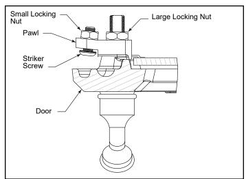
Figure 31 - Door latch adjustment.
