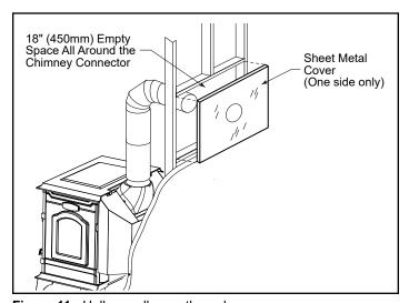
Figure 11 - Hollow wall pass-through.
