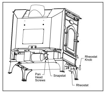
Figure 23 - Fan installation.
