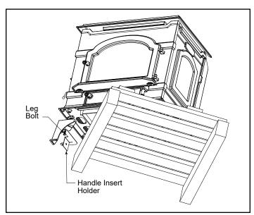
Figure 20 - Rotate stove on pallet to expose front left corner.
