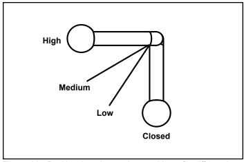
Figure 28 - Position the primary air control lever for different burn rates.
