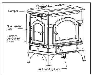
Figure 24 - The heater controls.
