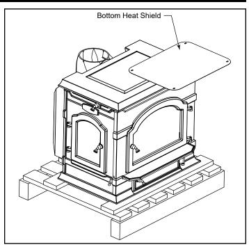
**Figure 19** - Remove bands holding stove to pallet and remove heat shield from to of stove.
