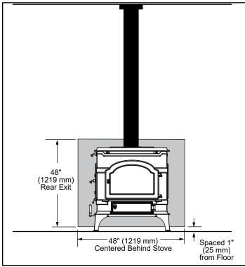
Figure 16 - Rear wall protection.
