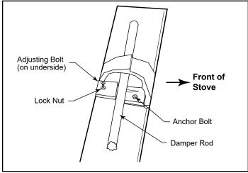
Figure 33 - Damper adjustment.
