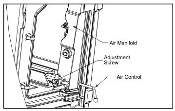
Figure 34 - Primary air control adjustment.
