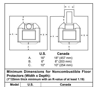
**Figure 12** - Be sure to follow exactly the minimum floor protection requirements on all four sides of the stove.
