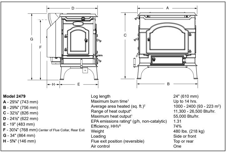
Figure 1 - Dutchwest Convection Heater specifications.
