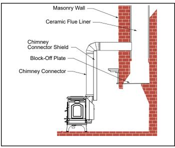
**Figure 8** - The connector enters flue above the fireplace. If the clearance between the chimney connector and either the mantel and/or the ceiling is inadequate, special protective shields will be required.
