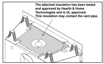
Figure 5.2 Top Insulation - CNXT4842IFT Models
