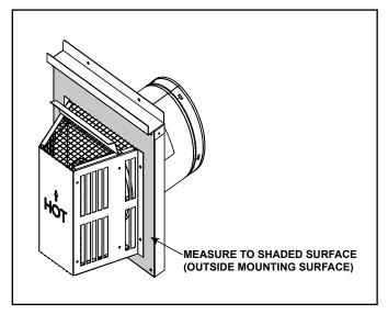
Figure 4.7 Measure to Outside Mounting Surface
