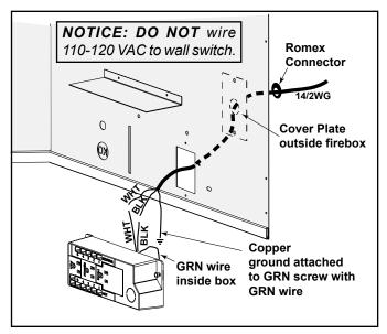
Figure 8.1 Junction Box Detail
