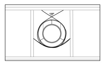
Figure 7.9 Securing Horizontal Pipe Sections
