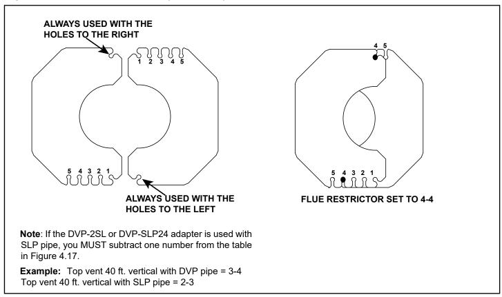
Figure 4.18 Setting the Flue Restrictor
