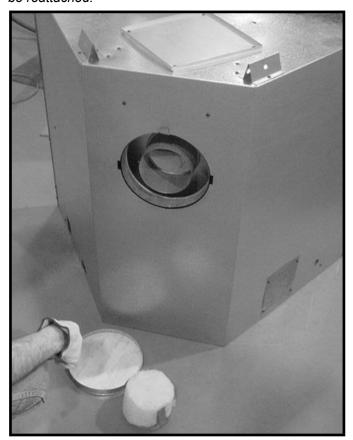
**Figure 6.10 (Generic Fireplace Shown)** Discard the vent cap, remove and discard the insulation basket.
