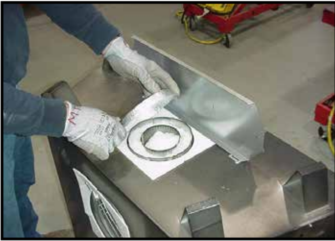
Figure 6.8 Remove the seal cap.
