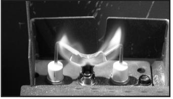
Figure 4.2 IPI Pilot Flame Patterns
