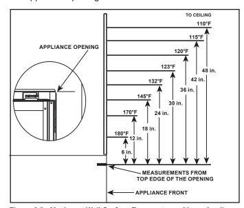
Figure 3.3. Maximum Wall Surface Temperatures Above Appliance
