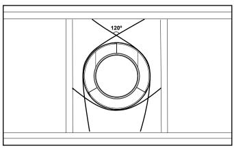
Figure 7.8 Securing Vertical Pipe Sections
