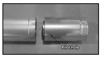
Figure 7.6 Slip Section Pilot Holes
