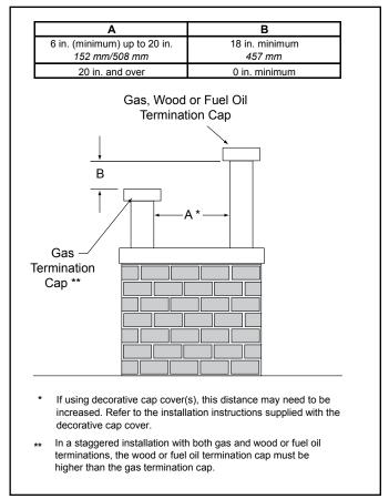
Figure 4.2 Staggered Termination Caps
