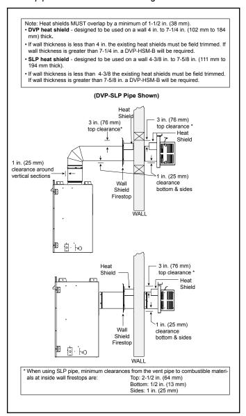
Figure 5.1 Horizontal Venting Clearances To Combustible Materials
