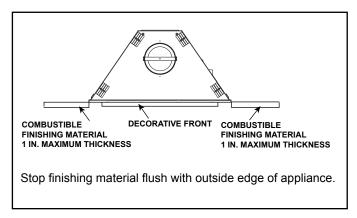
Figure 10.4 Combustible Finishing Material (Sides of appliance only. See Figure 10.1 for Combustible Mantel Clearances)
