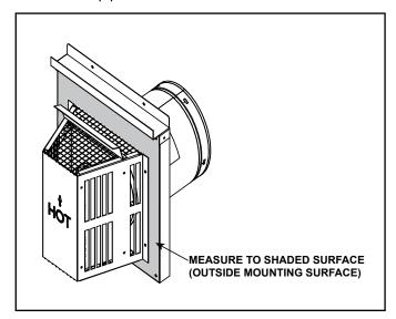
Figure 4.7 Measure to Outside Mounting Surface
