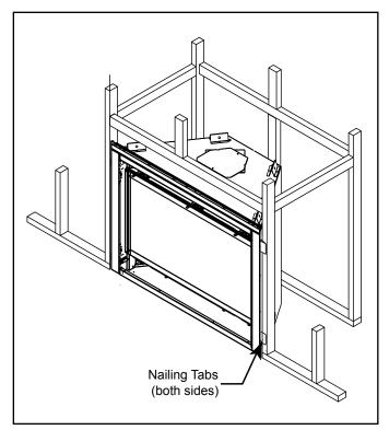
Figure 6.11 Proper Positioning and Securing of an Appliance
