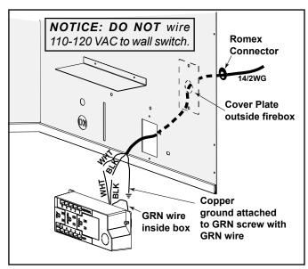
Figure 8.1 Junction Box Detail
