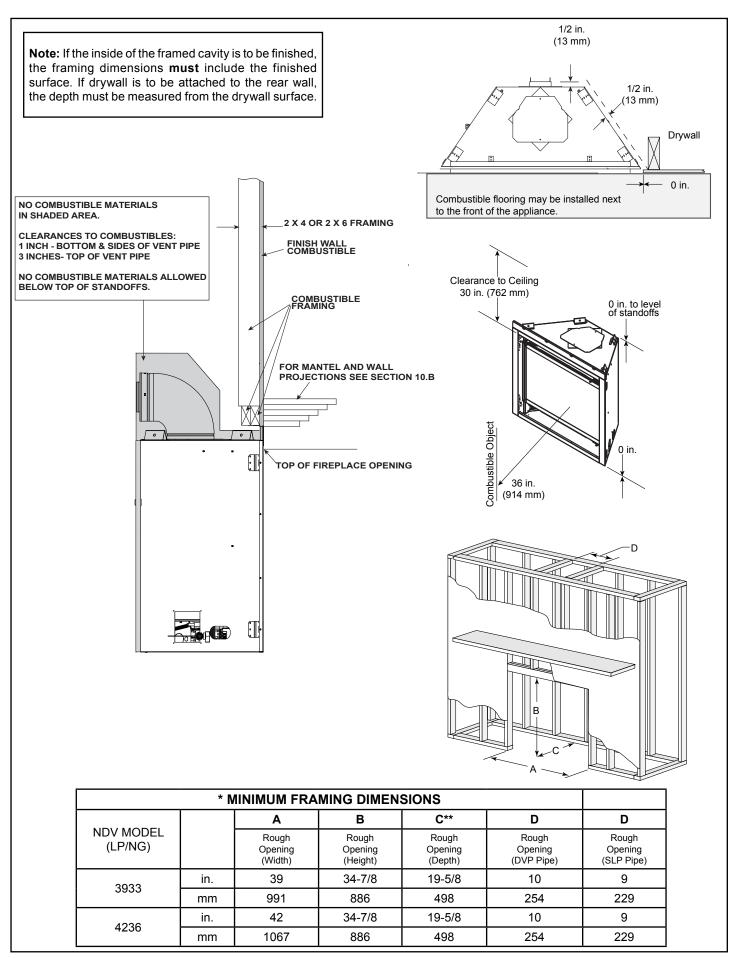
Figure 3.6 Clearances to Combustibles
