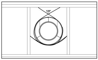
Figure 7.9 Securing Horizontal Pipe Sections
