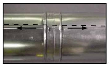
Figure 7.11 Align and Disassemble Vent Sections
