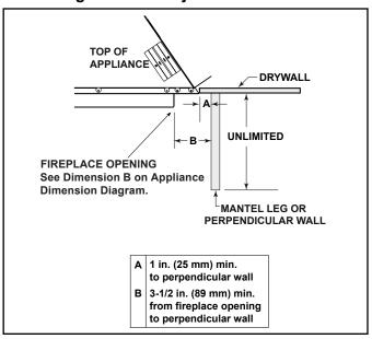
Figure 10.2 Mantel Leg or Wall Projections (Acceptable on both sides of opening)
