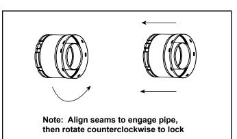
Figure 7.5 Adding Venting Components
