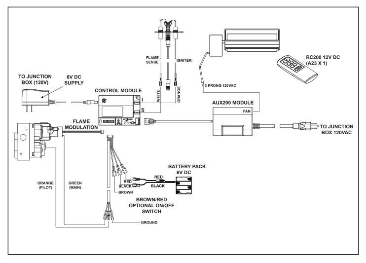
Figure 8.2 Intellifire Pilot Ignition (IPI) Wiring Diagram
