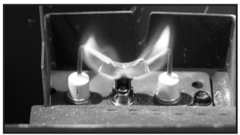
Figure 4.2 IPI Pilot Flame Pattern
