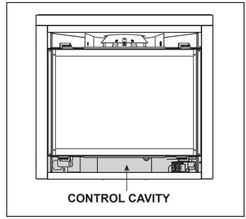
Figure 3.6 ON/OFF Switch/ Control Cavity Location
