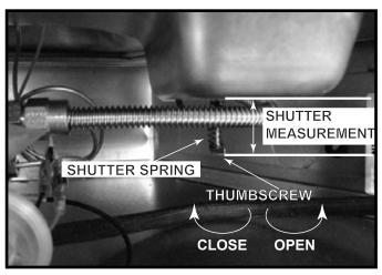
Figure 10.1 Adjusting Air Shutter
