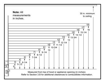
Figure 11.1 Minimum Vertical and Maximum Horizontal Dimensions of Combustibles
