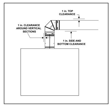
Figure 6.1 Horizontal Venting Clearances To Combustible Materials
