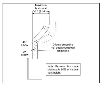
Figure 5.1 Maximum Horizontal Run Using 45° Elbows
