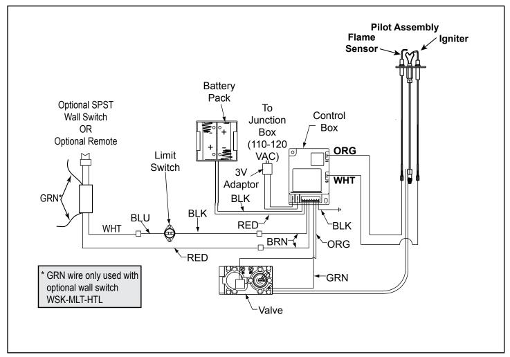
Figure 9.2 Intellifire Pilot Ignition (IPI) Wiring Diagram
