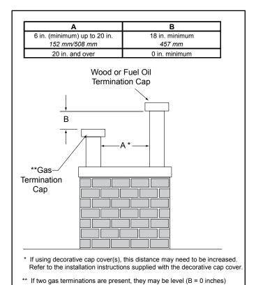
Figure 4.2 Staggered Termination Caps
