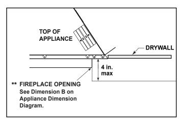
Figure 11.4 Non-Combustible Mantel Leg or Wall Projections (Acceptable on both sides of opening)
