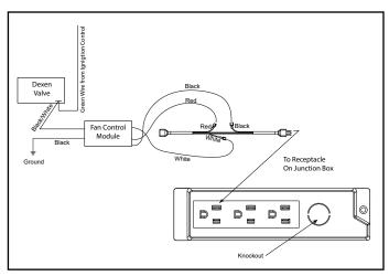
Figure 9.3 GFK21B or GFK4B Fan Kit Components
