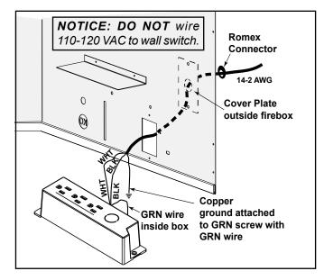
Figure 9.1 Junction Box Detail
