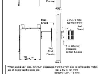
Figure 8.1 Horizontal Venting Clearances To Combustible **Materials**
