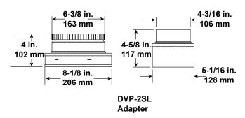
Figure 16.13 SLP Series Vent Components
