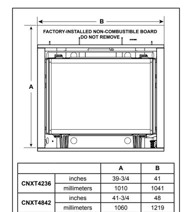
Figure 13.3 Noncombustible Facing Diagram
