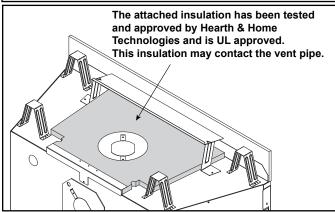
Figure 8.2 CNXT4842IT-D, CNXT4842IH-D Top Insulation
