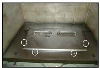
Figure 3.9 Remove Burner Skirt
