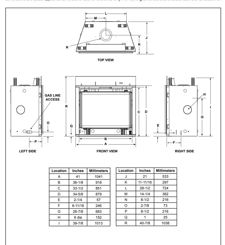
Figure 16.1 Appliance Dimensions-CNXT4236IT-D and CNXT4236IH-D Models
