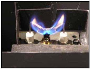
Figure 3.1 IPI Pilot Flame Patterns
