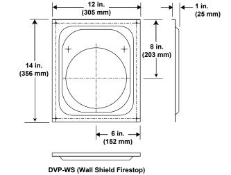
Figure 16.5 DVP Vent Components
