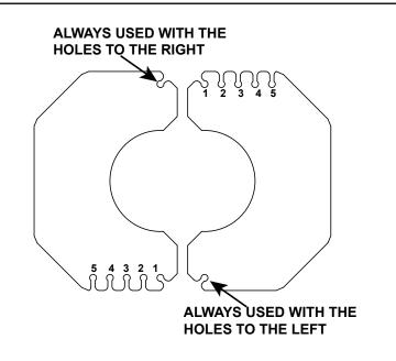
**Note**: If the DVP-2SL or DVP-SLP24 adapter is used with SLP pipe, you MUST subtract one number from the table in Figure 7.12.
