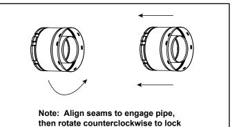
Figure 10.1 Adding Venting Components
