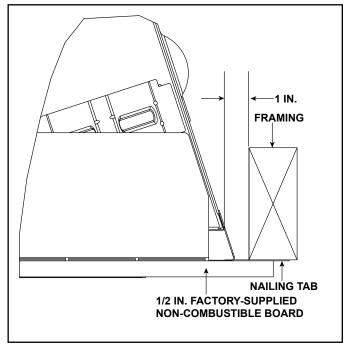
Figure 13.2 Front Side Finishing Detail
