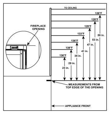
Figure 2.3. Wall Surface Temperatures Above Appliance
