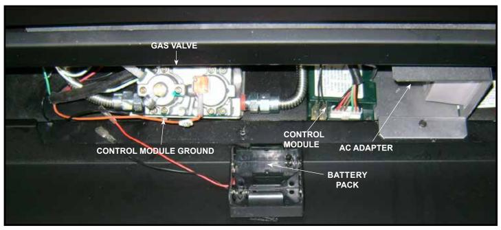
Figure 12.1 Valve Cavity
