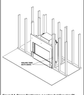
Figure 9.3 Proper Positioning, Leveling And Securing Of Appliance
