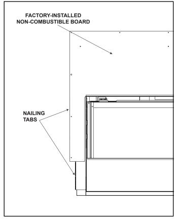
Figure 13.1 Nailing Tabs Installation Position
