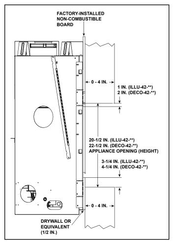
Figure 13.11 Inside Fit Method
