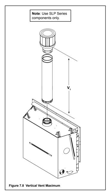
Exhaust restrictors are recommended for these vertically terminated products which have excessive draft. Exhaust restrictors will compensate for high draft, and restore visual flame height. If the vent configuration has a total vertical of 15-44 feet, an exhaust restrictor may be needed. The exhaust restrictor can be located in the appliance manual bag.
