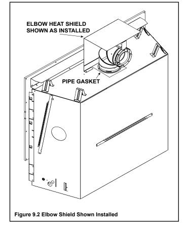
If venting with a 90 degree elbow directly off of the top of the appliance, the elbow heat shield must be repositioned as shown in Figure 9.2.
