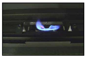
Figure 3.1 IPI Pilot Flame Pattern
