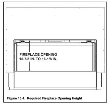
Verify that the lower cover panel is installed correctly, and that the fireplace opening height is between 15-7/8 in. and 16-1/8 in. See Figure 13.4.
