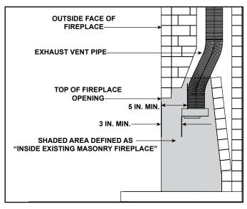
Figure 7.15 Existing Fireplace DV-46DVA-GCL Clearance Requirements
