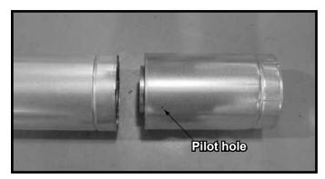
Figure 10.3 Slip Section Pilot Holes
