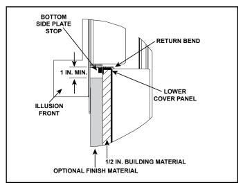
Figure 13.10. Illusion Front, Side View - Bottom Side Plate Installed Over Lower Cover Panel
