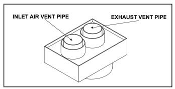
Figure 7.14 Coaxial/Colinear Appliance Adapter (DV-46DVA-GCL)
