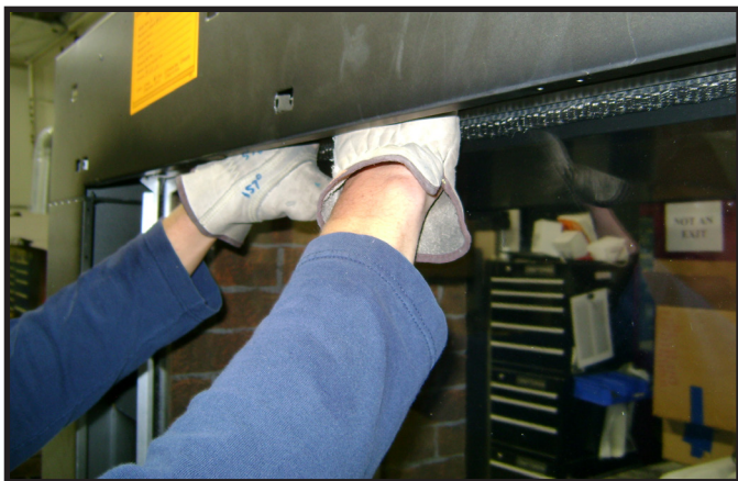
Figure 11.6 Top Glass Latch Access
