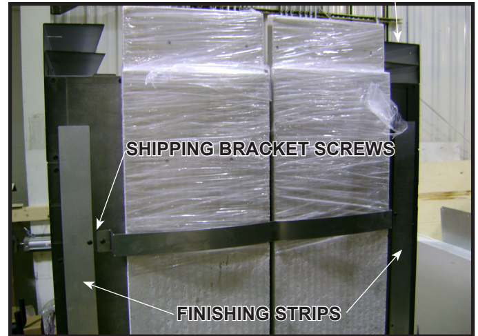
Figure 6.3 Shipping Brackets and Finishing Strip Locations.
