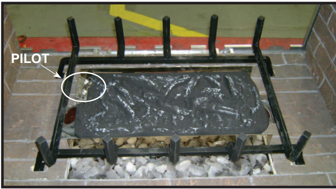
Figure 2. Burner and grate from front.
