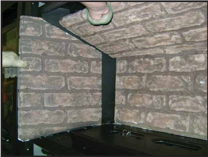
Figure 3.2 Top Refractory Removal
