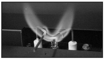
Figure 4.2 IPI Pilot Flame Patterns
