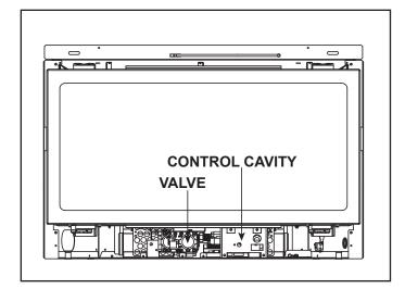
Figure 3.3 Control Cavity - Valve Location
