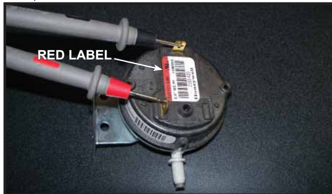
Figure 3.1. Test Exhaust Pressure Switch
