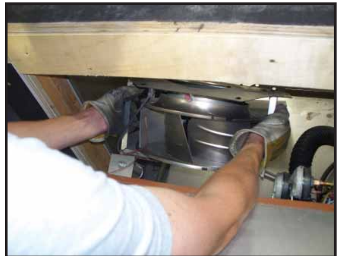
Figure 3.8. Remove Blower Assembly
