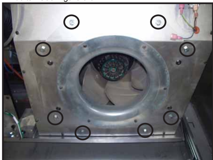
Figure 3.6. Remove Blower Assembly
