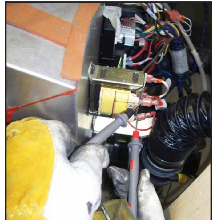
Figure 3.4. Test Terminals 4 and 5
