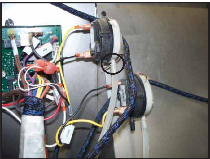
Figure 3.11. Disconnect Vacuum Tube
