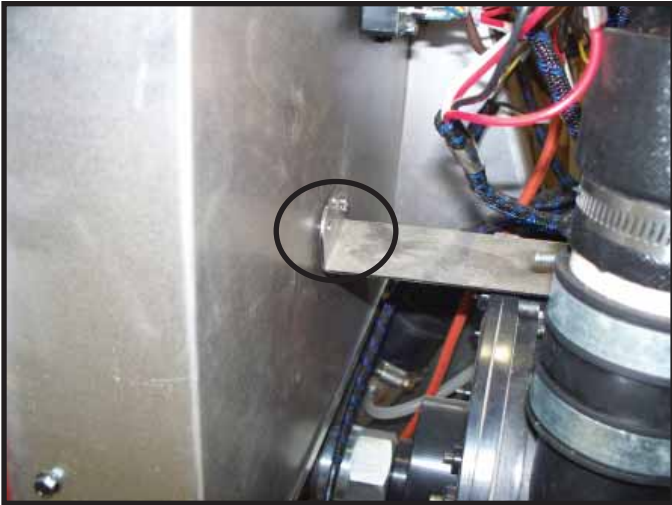
Figure 3.15. Remove Blower Assembly Bracket
