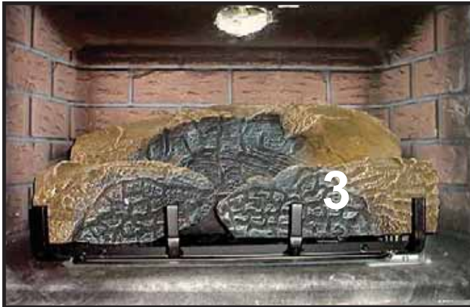
LOG #3 (SRV2032-703): Position log #3 by locating its slot over the tab on right front of the burner such that left end of log contacts log tab near the center of the burner.
