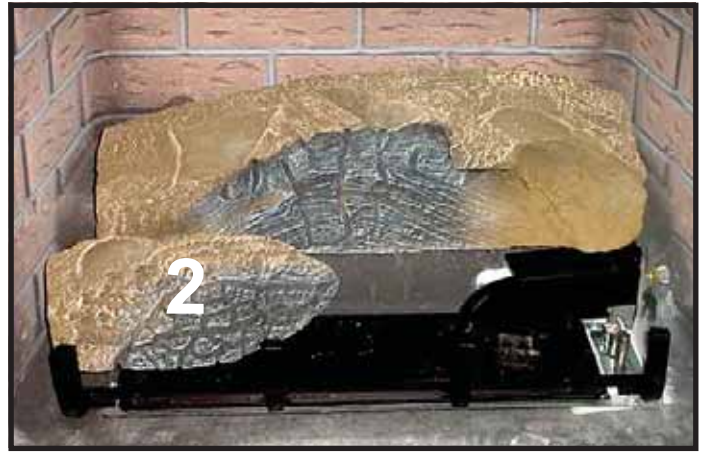
LOG #2 (SRV2032-702): Position log #2 by locating its slot over the tabs on left front of the burner.
