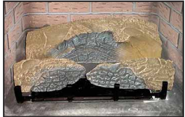
LOG #3 (SRV2032-703): Position log #3 by locating its slot over the tab on right front of the burner such that left end of log contacts log tab near the center of the burner.
