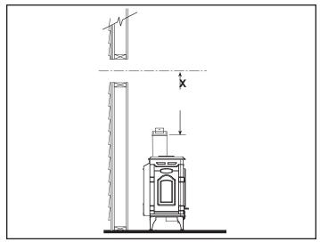
Figure 24 - Determine the vertical pipe length.
