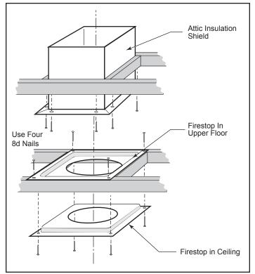
Figure 30 - Install firestops and attic insulation shield.
