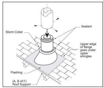
Figure 31 - Roof support and flashing.
