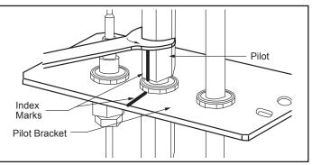
**Figure 55** - Remove pilot hood. (Your pilot may have a different appearance).
