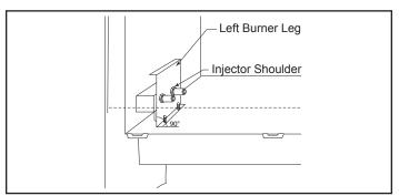
Figure 57 - Be sure to maintain 90° angle at left burner leg.
