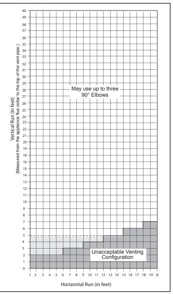
Figure 7 - Horizontal vent termination window.
