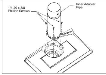
Figure 20 - Simpson DuraVent - install inner adapter pipe.
