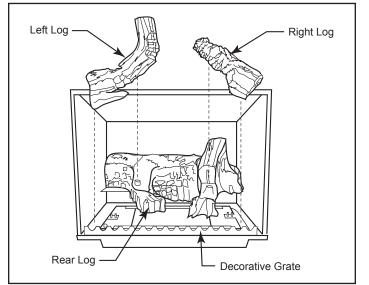
Figure 34 - Install the back, left and right logs.
