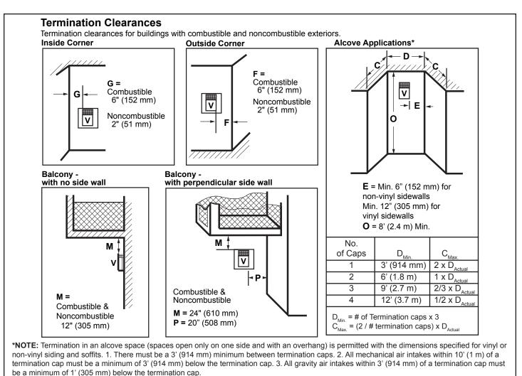
Figure 10 - Termination clearances.
