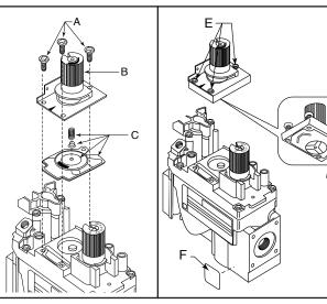
**Figure 51 -** Remove mounting screws, pressure regulator tower and spring and diaphragm assembly.
