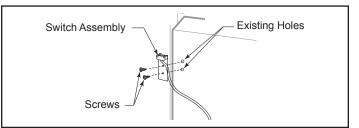
Figure 41 - Attach switch assembly to rear shroud.
