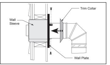
Figure 26 - Install the horizontal pipe and wall plate parts.
