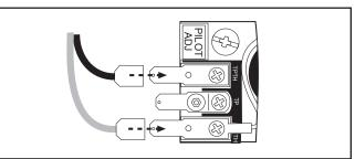
Figure 42 - Attach switch wires to valve.
