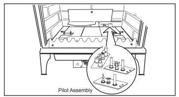
Figure 46 - Pilot assembly location.
