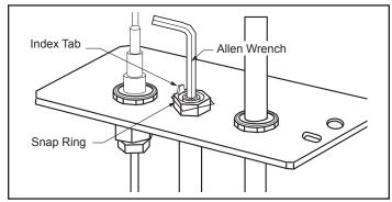
Figure 54 - Remove pilot orifice.
