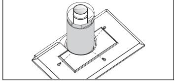
Figure 21 - Simpson DuraVent - install outer adapter pipe.
