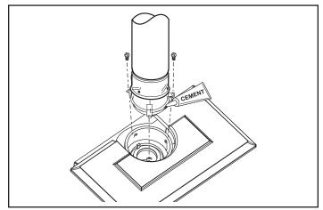
Figure 18 - Attach inner assembly to flue collar.
