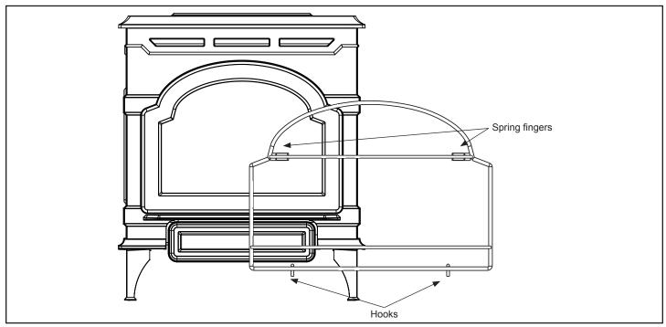
Figure 45 - Safety Barrier Installation
