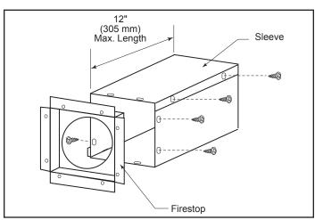
Figure 23 - Assemble the wall sleeve and firestop.
