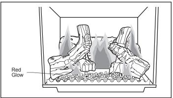
Figure 61 - Correct flame pattern.
