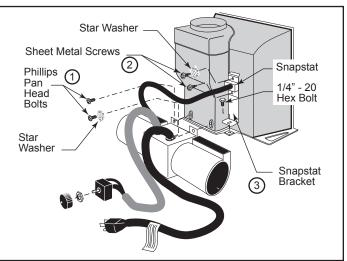
Figure 14 - Attach the fan assembly and the snapstat.
