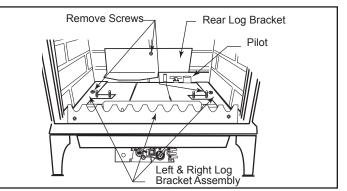
Figure 37 - Remove rear log bracket and left and right log bracket assembly.
