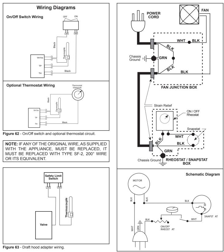
Figure 64 - Fan circuit.
