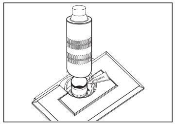
Figure 33 - Install draft hood adapter.
