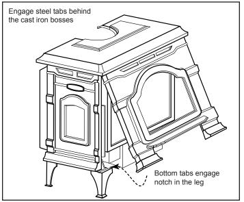
Figure 44 - Install the - front plate.
