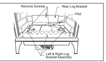
**Figure 50 -** Remove rear log bracket and left and right log bracket assembly.
