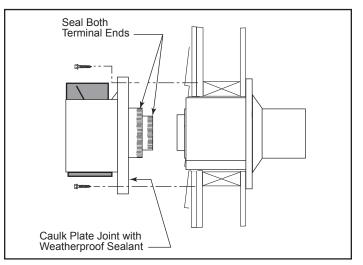
Figure 27 - Install the vent terminal.
