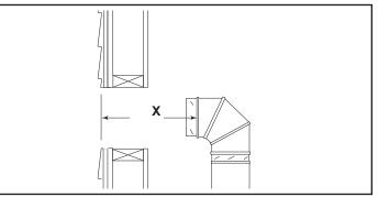
Figure 25 - Measure the horizontal length.
