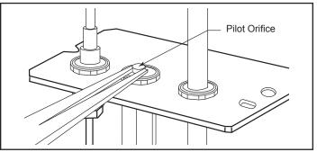
Figure 56 - Remove pilot orifice.
