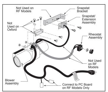
Figure 12 - Fan kit components.
