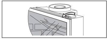
Figure 59 - Release the latches to release the glass frame.
