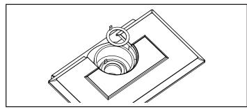
**Figure 16** - Install the restrictor plate only if required for the venting configuration. Refer to Page 9.
