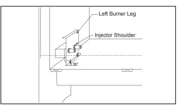
Figure 40 - Be sure to maintain 90° angle at left burner leg.
