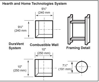
Figure 22 - Locate vent opening
