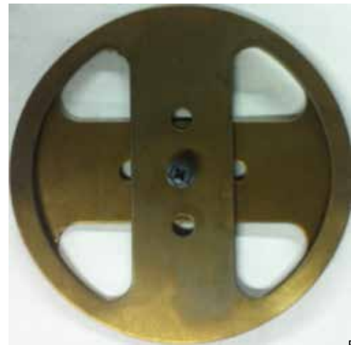
Figure 41 – Flue Restrictor Set at Maximum Restriction
