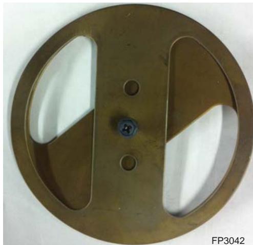
Figure 43 – Flue Restrictor Set at Medium Restriction
