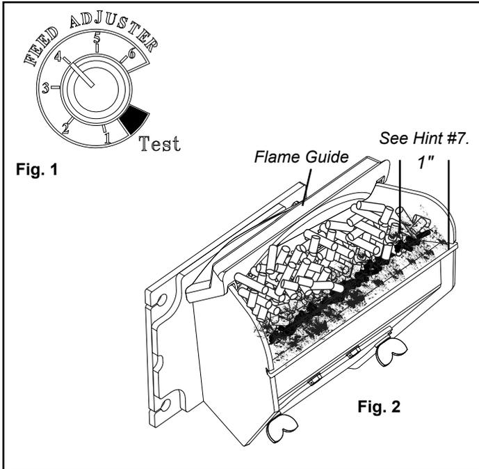
1. Fines are small pieces of broken pellets (sawdust). Fines do not flow easily and often build up on the hopper funnel bottom angles. These fines can be pushed into the feeder opening and then fill the hopper with pellets. As the system works, they will be burned.
