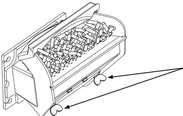
Loosen these two wing screws for access to clean the air passage and igniter.
