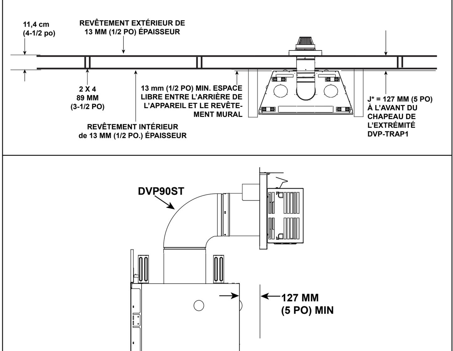
Figure 3.9 Exception DVP-TRAP1 (construction 2 x 4)
