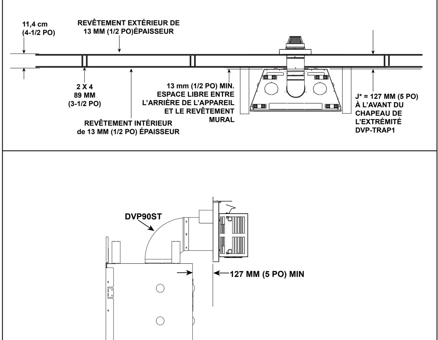
Figure 3.8 Exception DVP-TRAP1 (construction 2 x 4)
