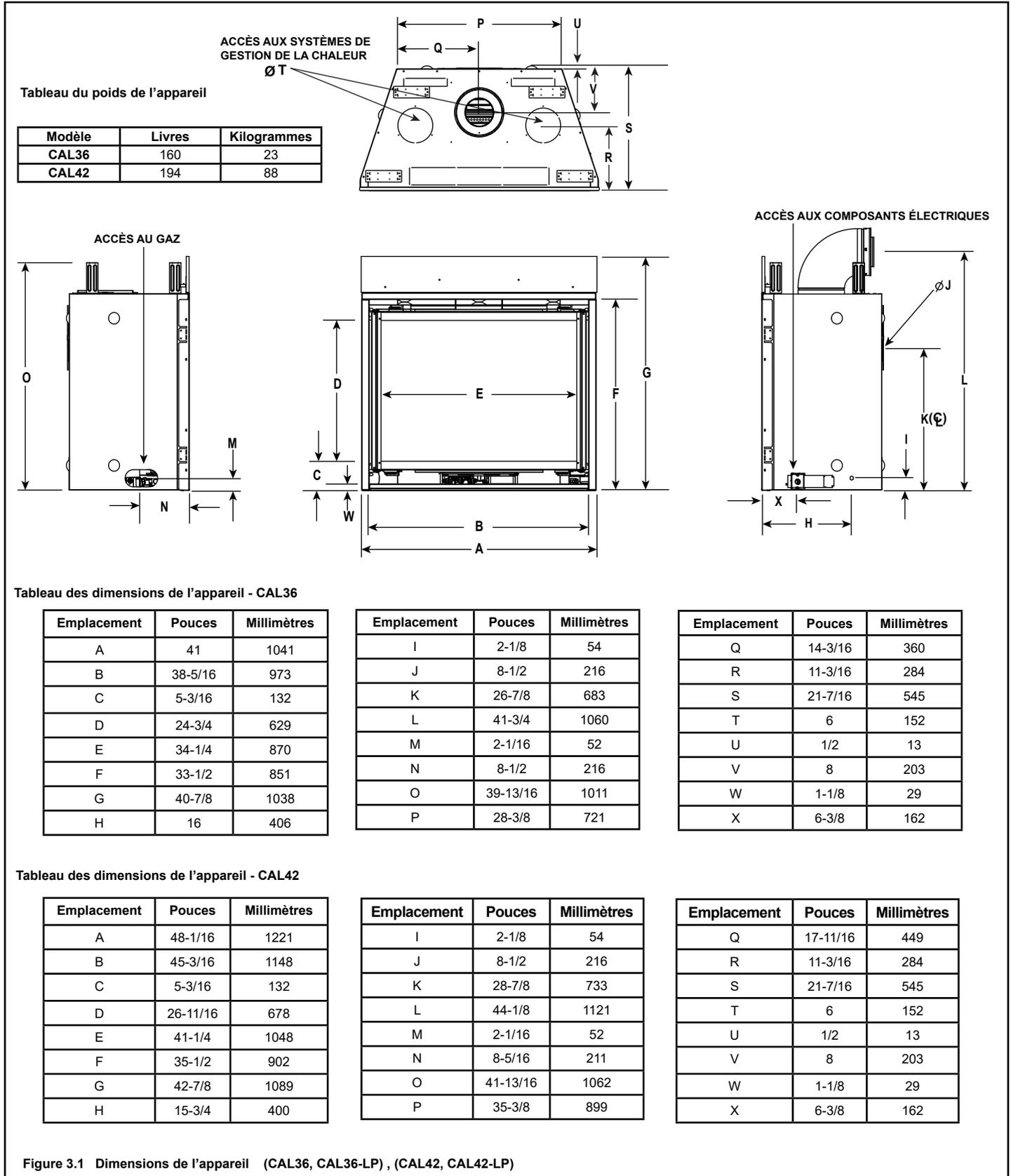
Figure 3.1 Dimensions de l'appareil (CAL36, CAL36-LP), (CAL42, CAL42-LP)
