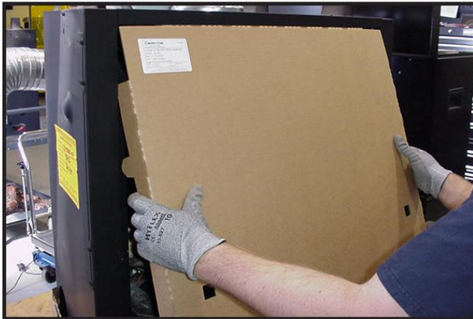
Figure 11.5 Installation de l'anti-projection
