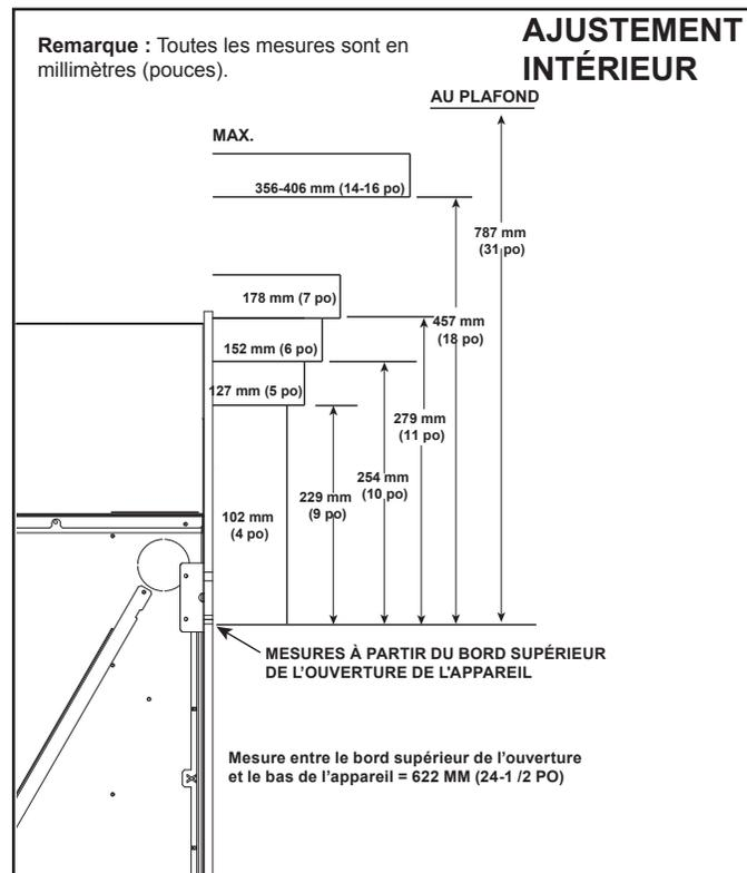
Figure 10.15 Minimum vertical et maximum horizontal
