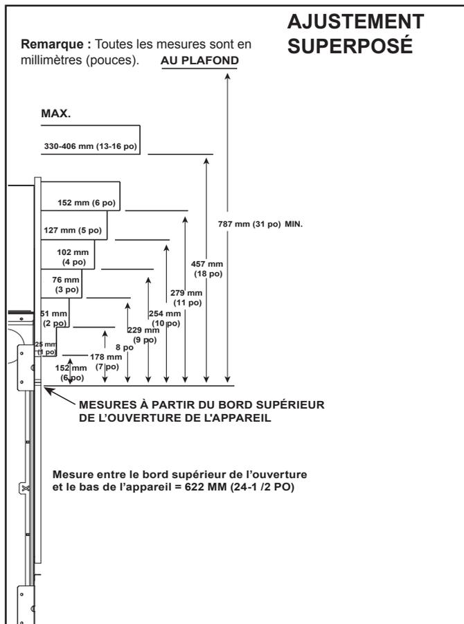
Figure 10.14 Minimum vertical et maximum horizontal
