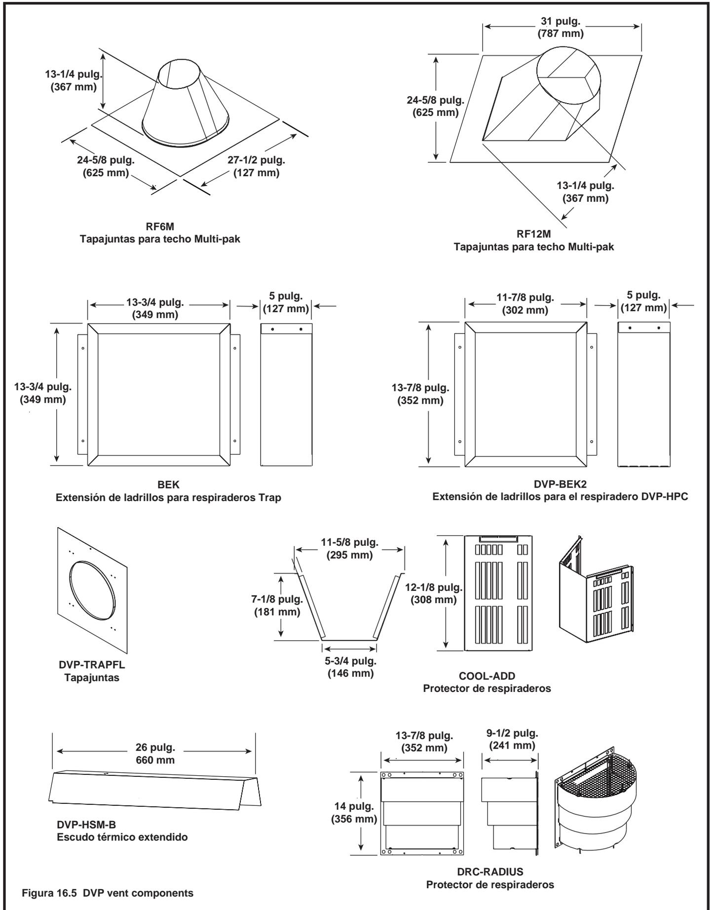
Figura 16.5 DVP vent components
