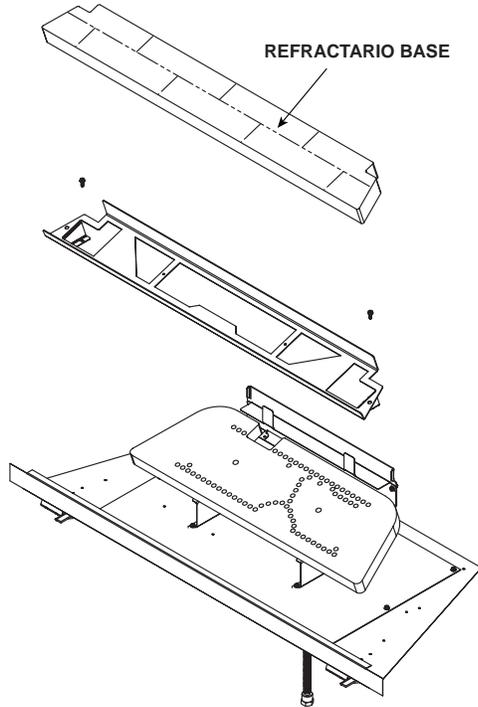
Figura 3.5 Retire el refractario base
