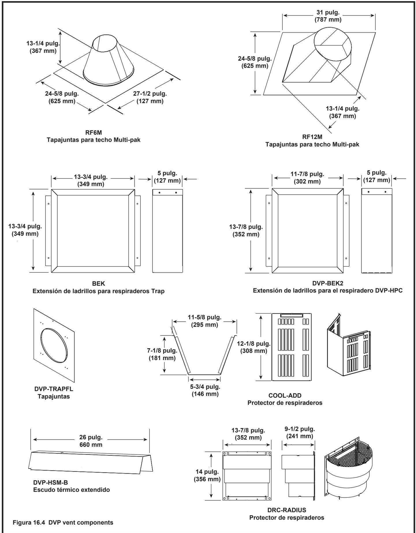
Figura 16.4 DVP vent components
