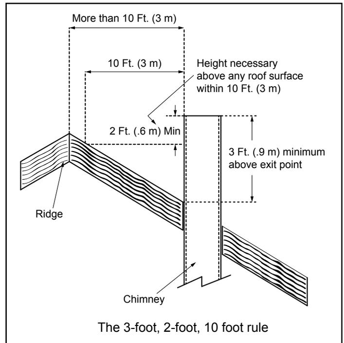
Codes require that solid-fuel chimneys extend 3 ft (0.9 m) above the point at which they exit from the roof, provided that no part of any structure is within the top of the chimney, then the chimney must extend 2 ft (6 m) above the highest point with the 10 ft (3 m) radius top height. If there is not ten feet of clearance from the top of the chimney, then the chimney must extend 2 ft (6 m) above the highest point with the 10 ft (3 m) radius.
