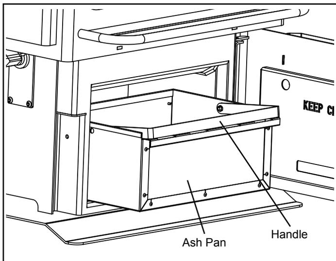
**Disposal of Ashes.** The TLC 2000 was designed to provide access to the ash pan without the need for opening the main door. Wearing heavy protective gloves, open the ash door and remove the ash pan by pulling it forward by the handle. Close the ash door before taking the ashes outside for safe disposal.
