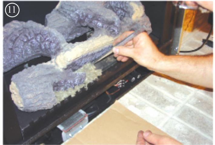
Place rock wool on burner as shown above. The wool should be placed loosely and lightly. This wool forms the glowing ember bed and will look different depending on placement. Reinstall the glass door assembly and close the latches.
