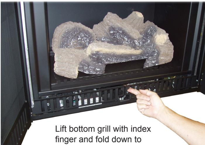
Lift bottom grill with index finger and fold down to access controls
