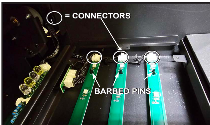
Figure 19 LED Connectors and Barbed Pins
