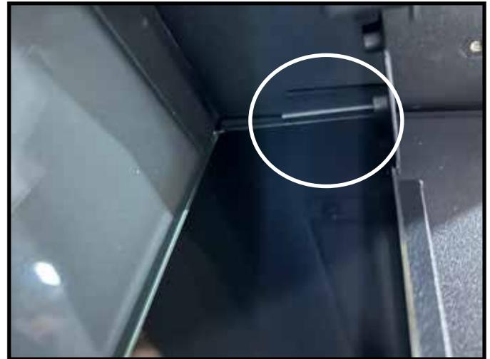
Figure 12 Upper Bracket on Side Panel
