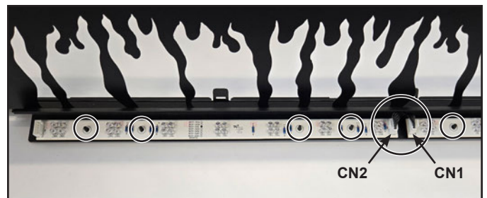
Figure 20 LED Connectors and Plastic Retainers
